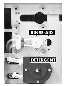
The 401HT pumps are located on the left-side behind the lower front panel of the dishwasher.
