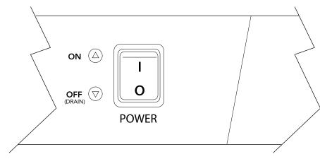
Place the Power Switch in the OFF/(DRAIN) position
