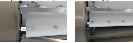
By removing both scrapers, the whole machine is exposed and ready to be cleaned.
