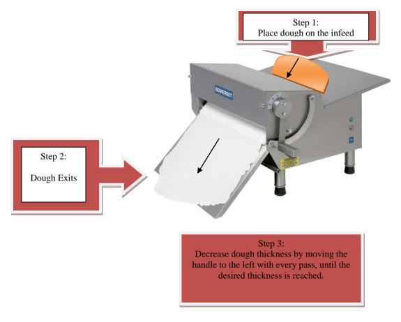
If the dough tears or the machine makes a thumping sound, this indicates that the dough is too thick to go through that particular setting of the rollers or the dough is too cold and stiff and requires longer rest period before use.
