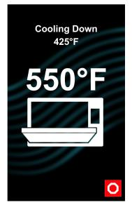
"Cooling Down" screen appears and stays on until oven temperature is below 200°F (95°C)
