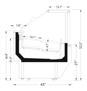
\* Customizable options available; \* Multiple shelves available; \* All measurements are approximates; \* Specifications are subject to change without notice; \* All equipment are designed to operate in a controlled environment below 75°F (+24°C) temperature and HR 55% relative humidity;
