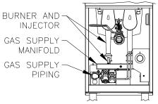
ADJUST GAS SUPPLY COMPONENTS IF NECESSARY. ENSURE THAT THE INJECTORS ARE PERPENDICULAR TO THE MANIFOLD AND PARALLEL TO THE BURNERS.
