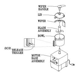
**STEP #2.** Place the blade on the motor shaft. It may be necessary to rotate the blade until it falls into place on the motor shaft. When the "S" blade is in the correct position the lower blade should be resting just off the bottom of the bowl.
