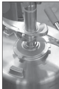
12) Push down blade assy, stop when hits motor shaft
