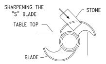
4. With the other hand hold the stone at a 30 degree angle
