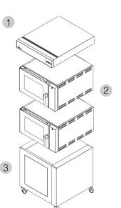
2 Two KX-5+H ovens Height: 535 mm/oven. Capacity: 5 trays (60 x 40 cm)/oven o 5 trays (66 x 46 cm)/oven. Total capacity: 10 trays.
